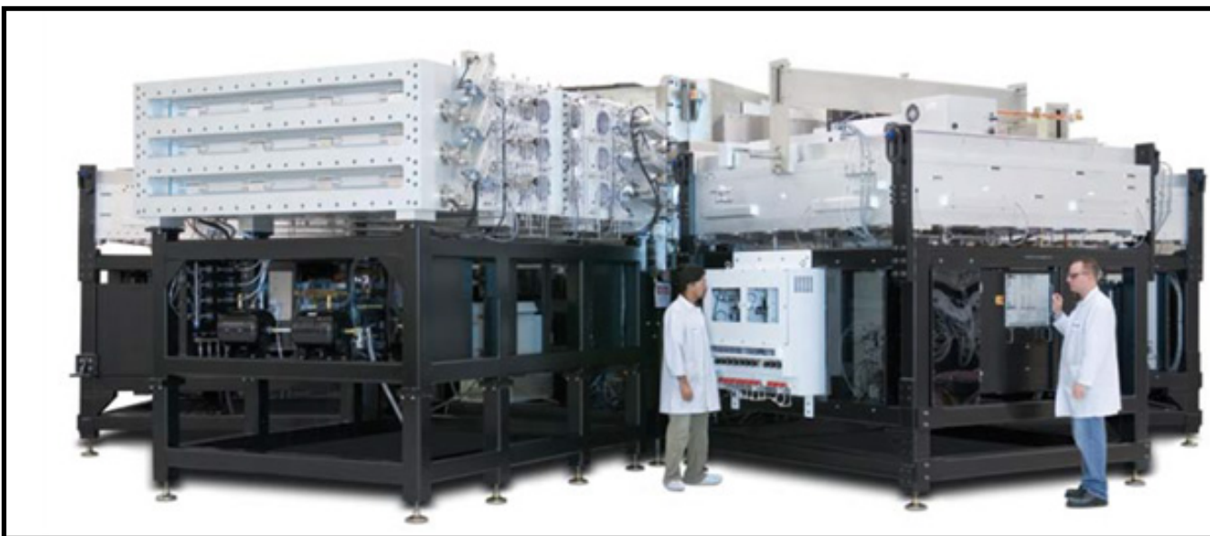
Figure 6.1: AKT PECVD System used for a-Si:H Deposition Ref: Applied Materials ( www.appliedmaterials.com )
