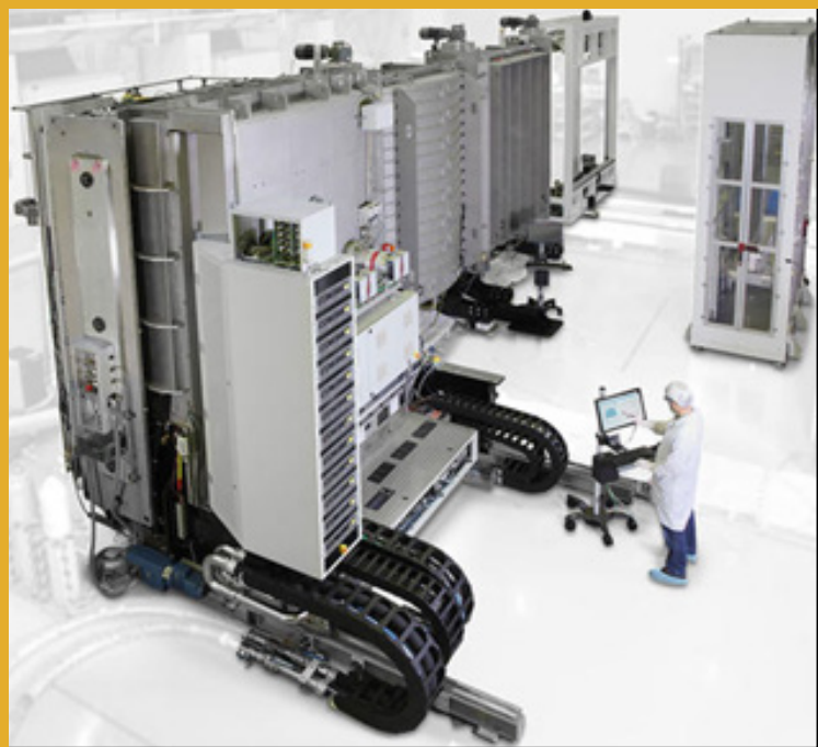
Figure 6.3: AKT PVD system used for IGZO deposition Ref: Applied Materials ( www.appliedmaterials.com )
